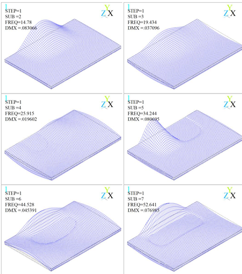
Figure 68. The 1st - 6th mode shapes for the 1/3 unsymmetrical delaminated model.
