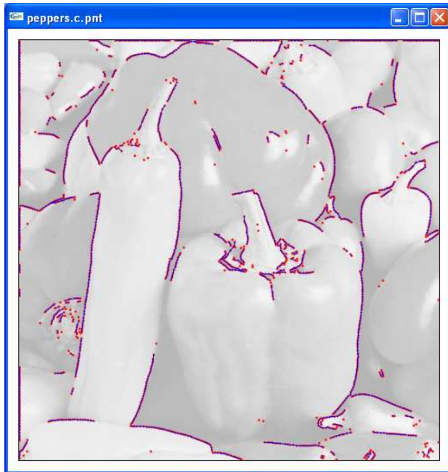
Fig. A.7: Command: ./make peppers.c.l.show ST=0.3 IMG=peppers.ppm . 167 paths and 1721 points
