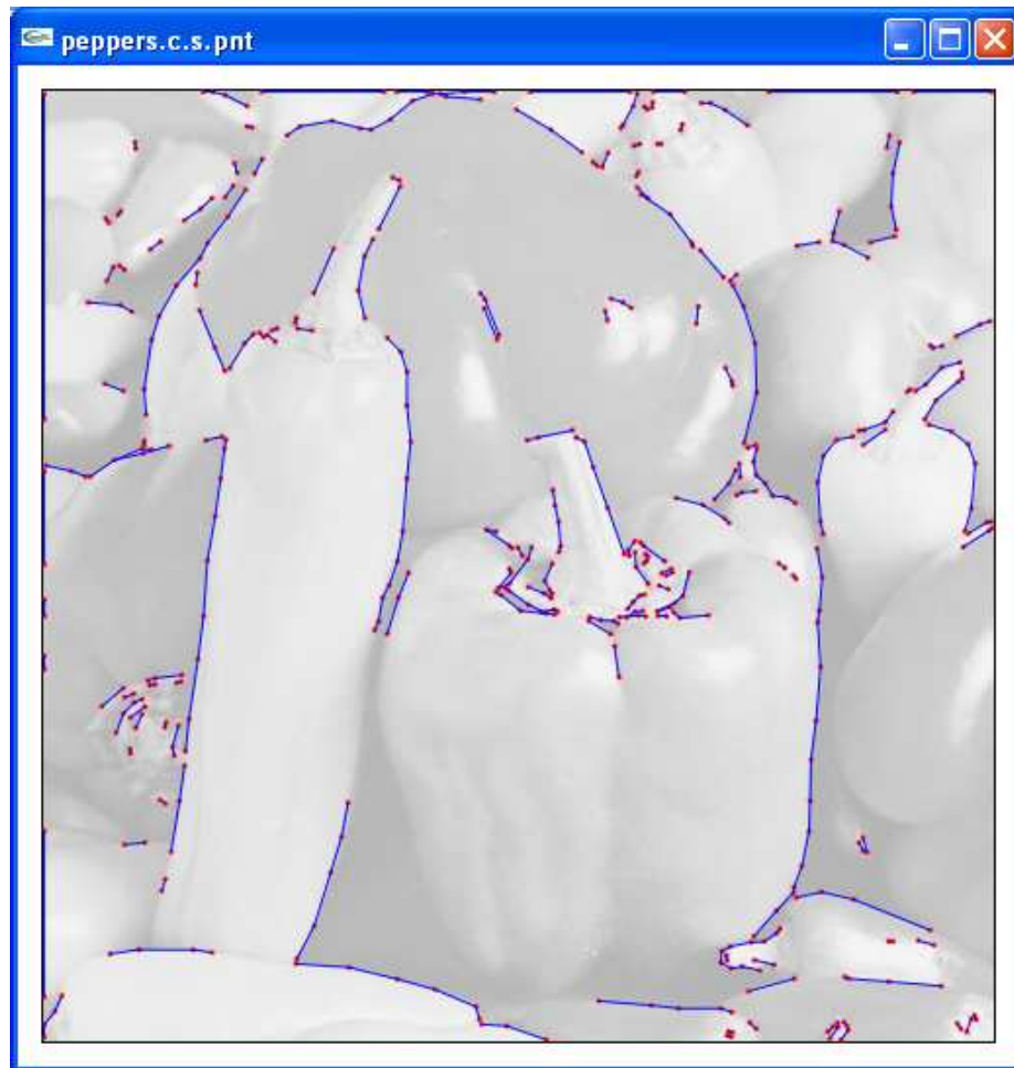
Fig. A.8: Command: ./make peppers.c.s.show ST=0.3 IMG=peppers.ppm . 167 paths and 498 points
