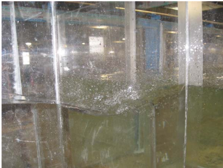
Figure 13. Hydraulic jump in the throat. At a flow rate of 1.50 cfs and submergence at 87%, the water is flowing from the canal back into the throat. The main flow direction is from left to right with the hydraulic jump moving against the main flow.
