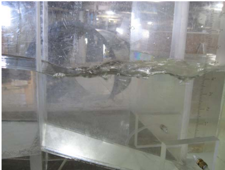
Figure 15. Secondary unstable flow. At a flow rate of 0.50 cfs and submergence at 84%, the flow conditions are unstable. Picture 2 of 2 with water flowing left to right. The two pictures are taken 5 seconds apart and demonstrate unstable hydraulic conditions experienced during laboratory testing.
