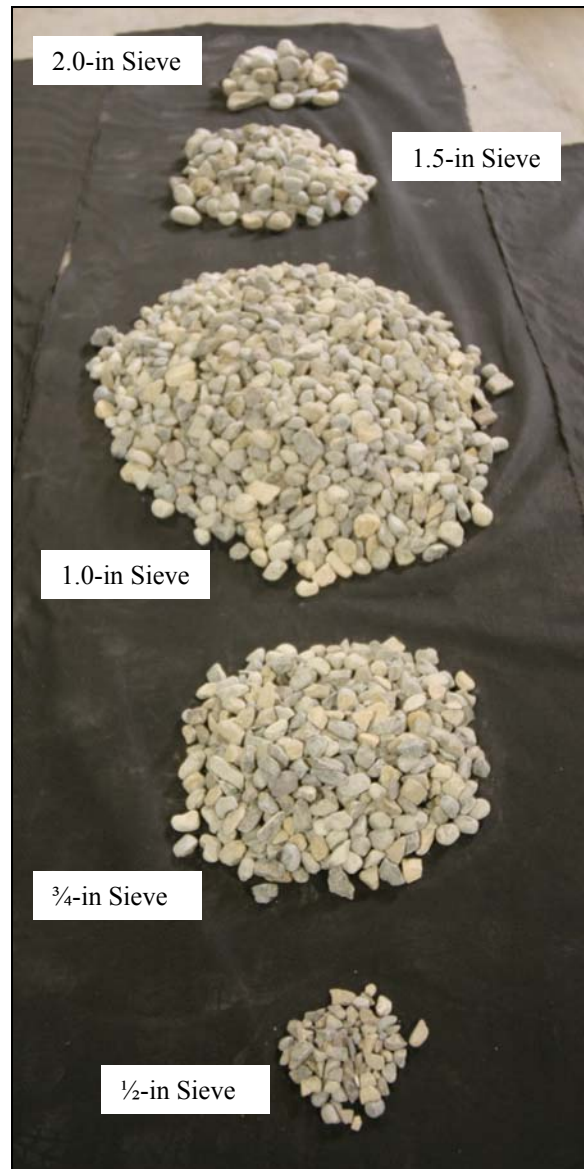
Figure G3. Sieve distribution of 2-inch cobble substrate
