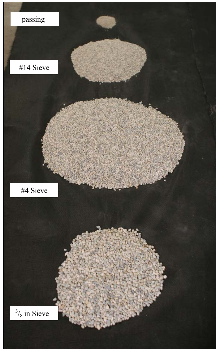
Figure G1. Sieve distribution of pea gravel substrate
