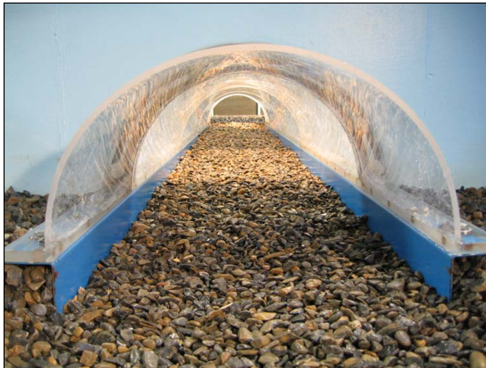
Figure 48. Scour of 0.75-inch angular gravel looking upstream from exit, 1 H_w/D .
