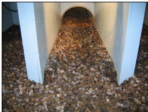
Figure 8. 0% Contraction with headwall.
