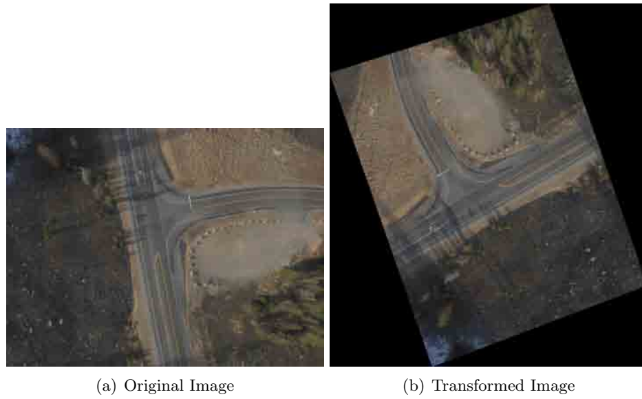
Fig. 4.12: Perspective transformation example.
