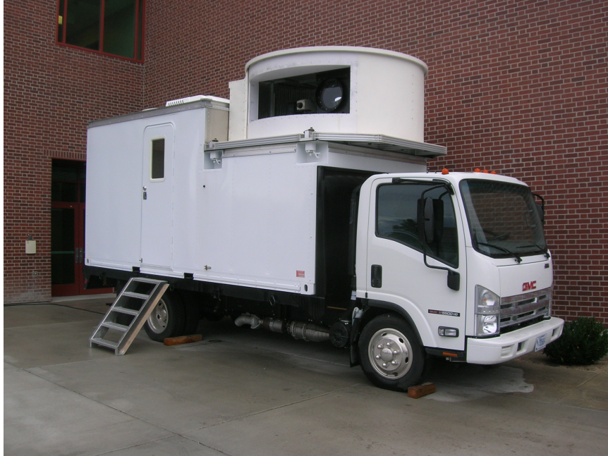
(a) The ELT aperture can be seen at the right side in the turret behind the cab.
