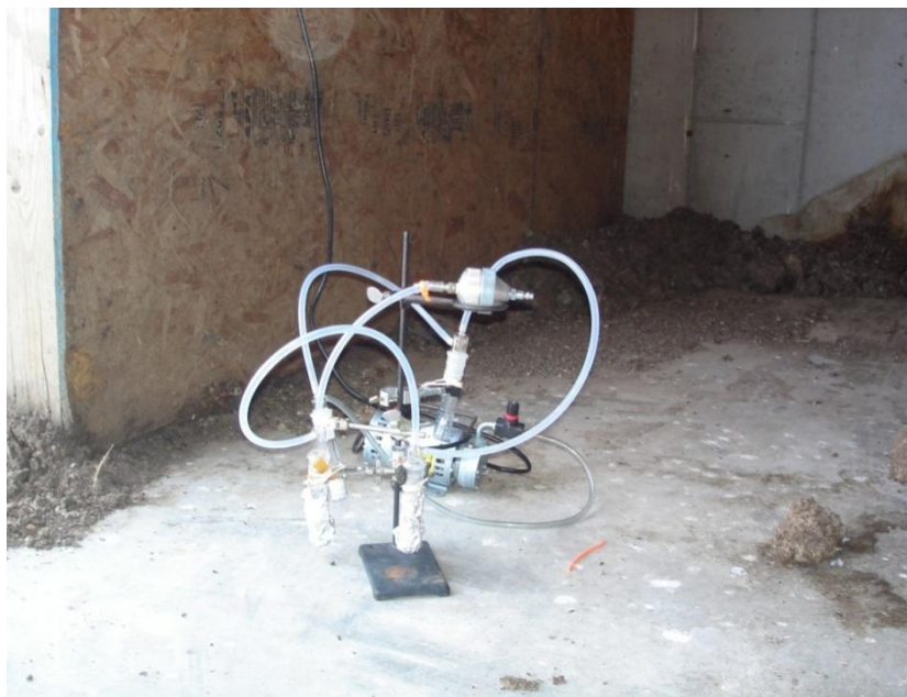
Fig. 3. Impinger sampling train at north door of the manure barn on October 6 th , 2008.
