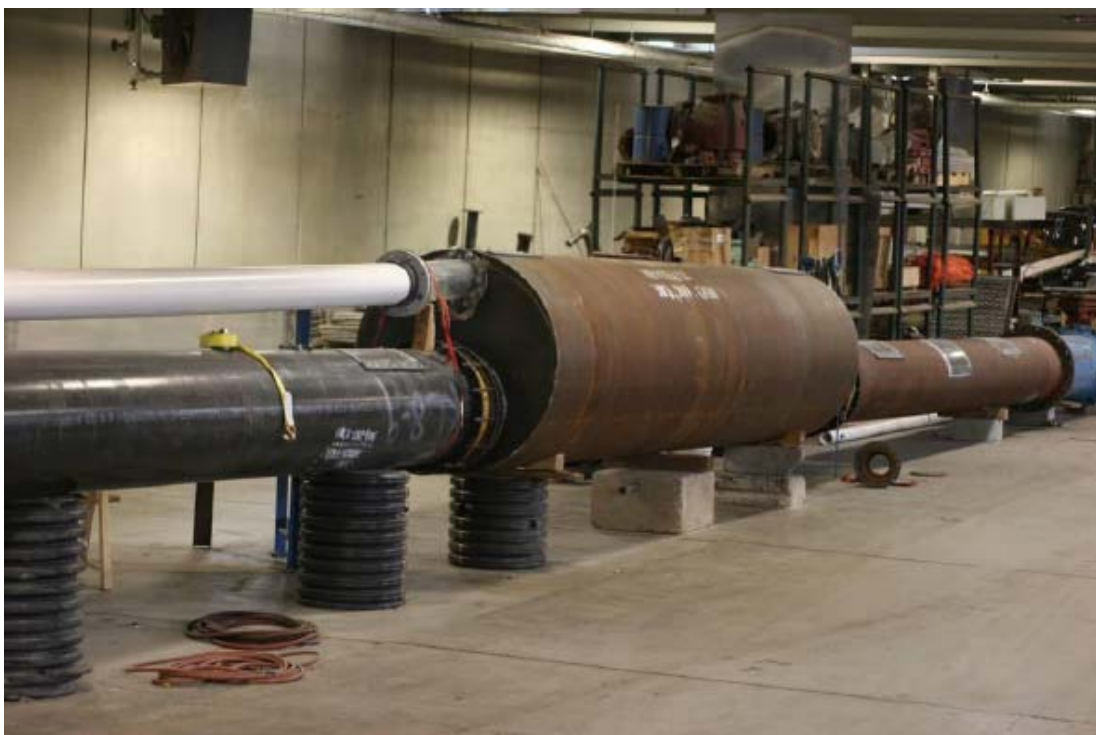
Figure 14 24-inch model with air capture chamber and vent
