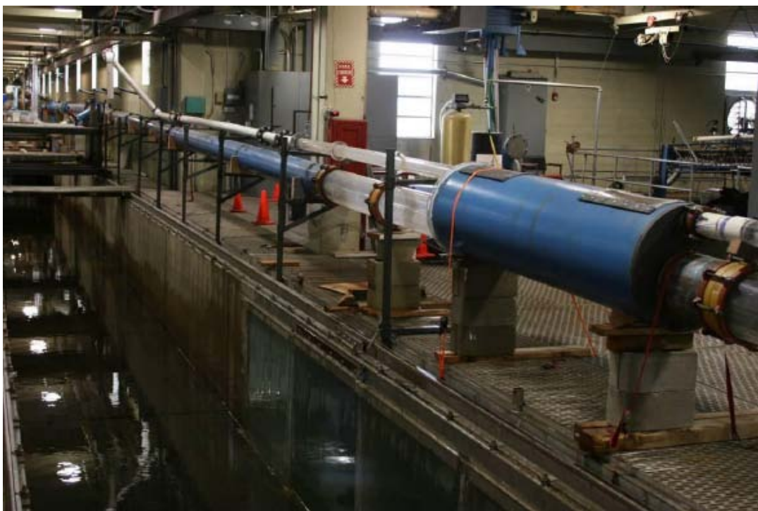
Figure 16 12-inch pipe model
