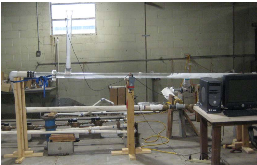
Figure 19 3-inch acrylic pipe and air intake just downstream of flow nozzle
