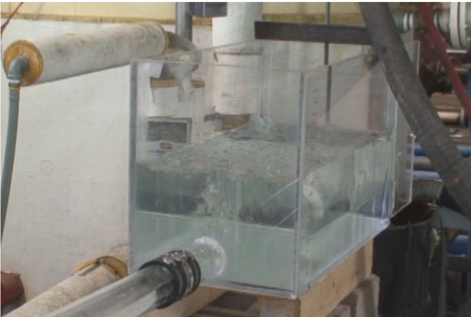
Figure 22 Rectangular Open Tank on the 3-inch acrylic pipe
