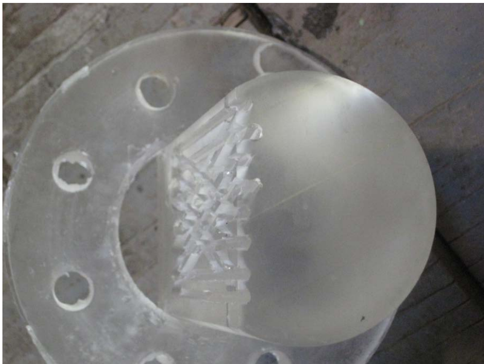
Figure 23 Roughened flow nozzle for rough water surface tests in 3-inch pipe
