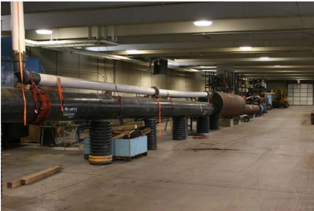
Figure 13 24-inch pipe model
