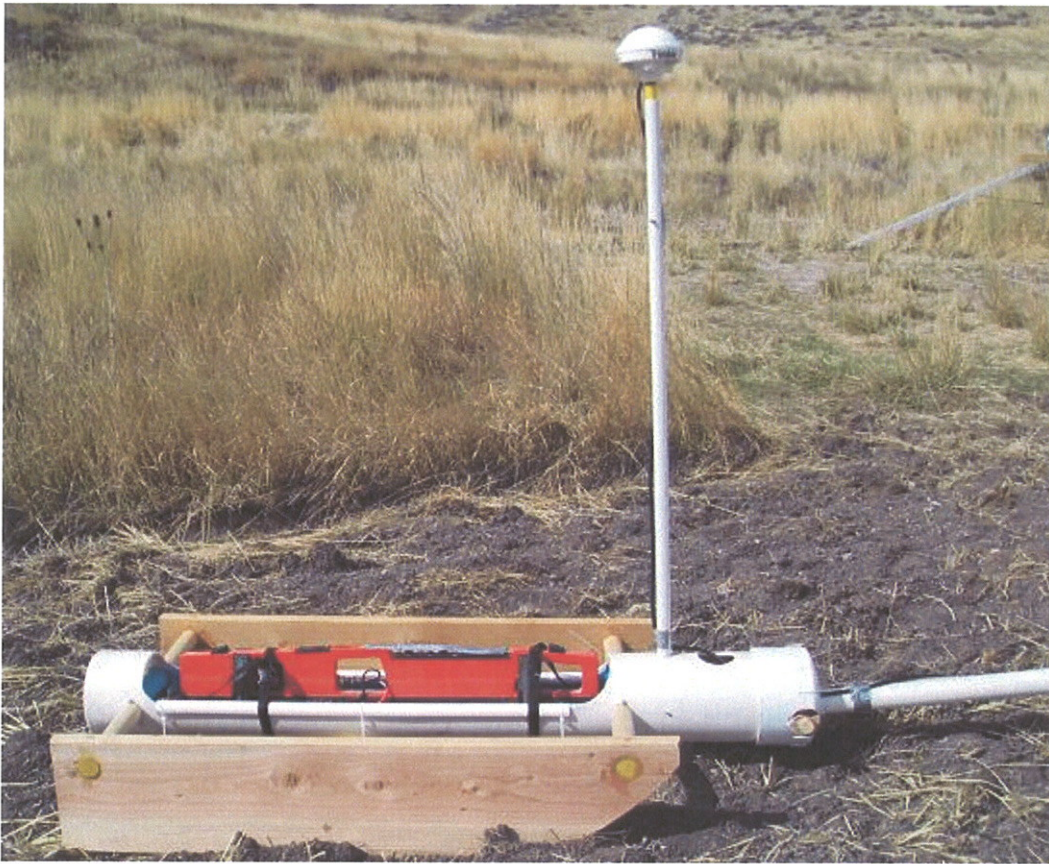
Fig. 3.3. The mobile EC_a measurement apparatus with the EM-38 DD prepared for a survey.
