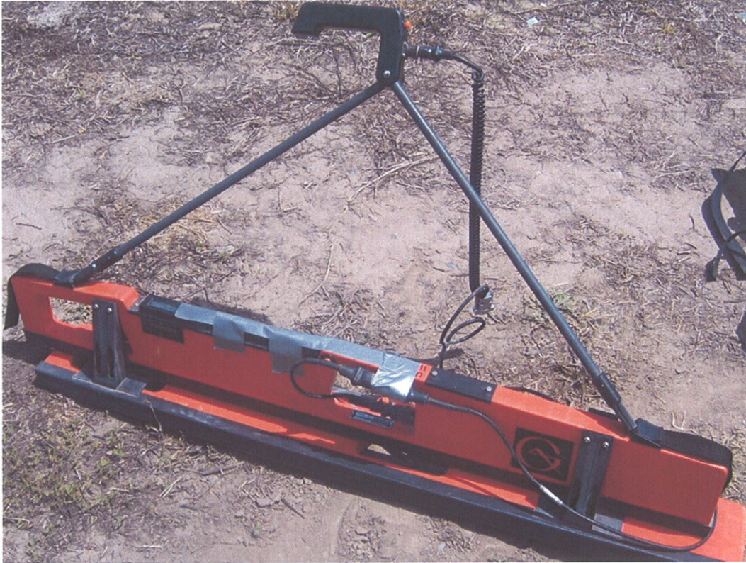
Fig. 3.2. The EM-38 DD prepared for a manual survey.
