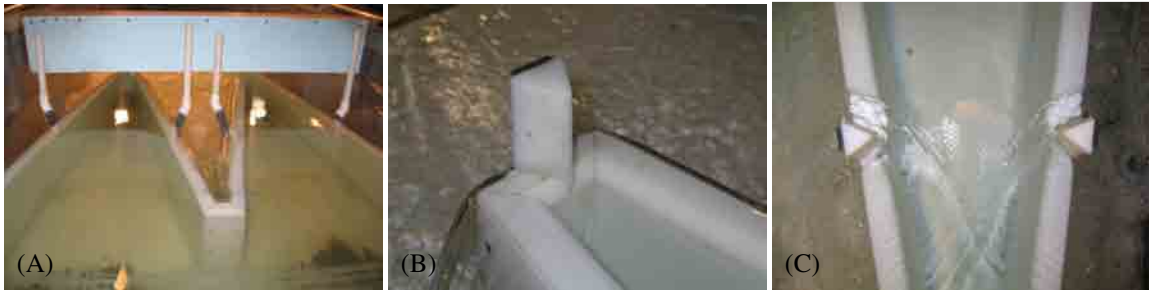
Fig. 6-6. Aeration tube apparatus for N = 2 (A) and nappe breakers located on the downstream apex (B) and on the sidewall (C)
