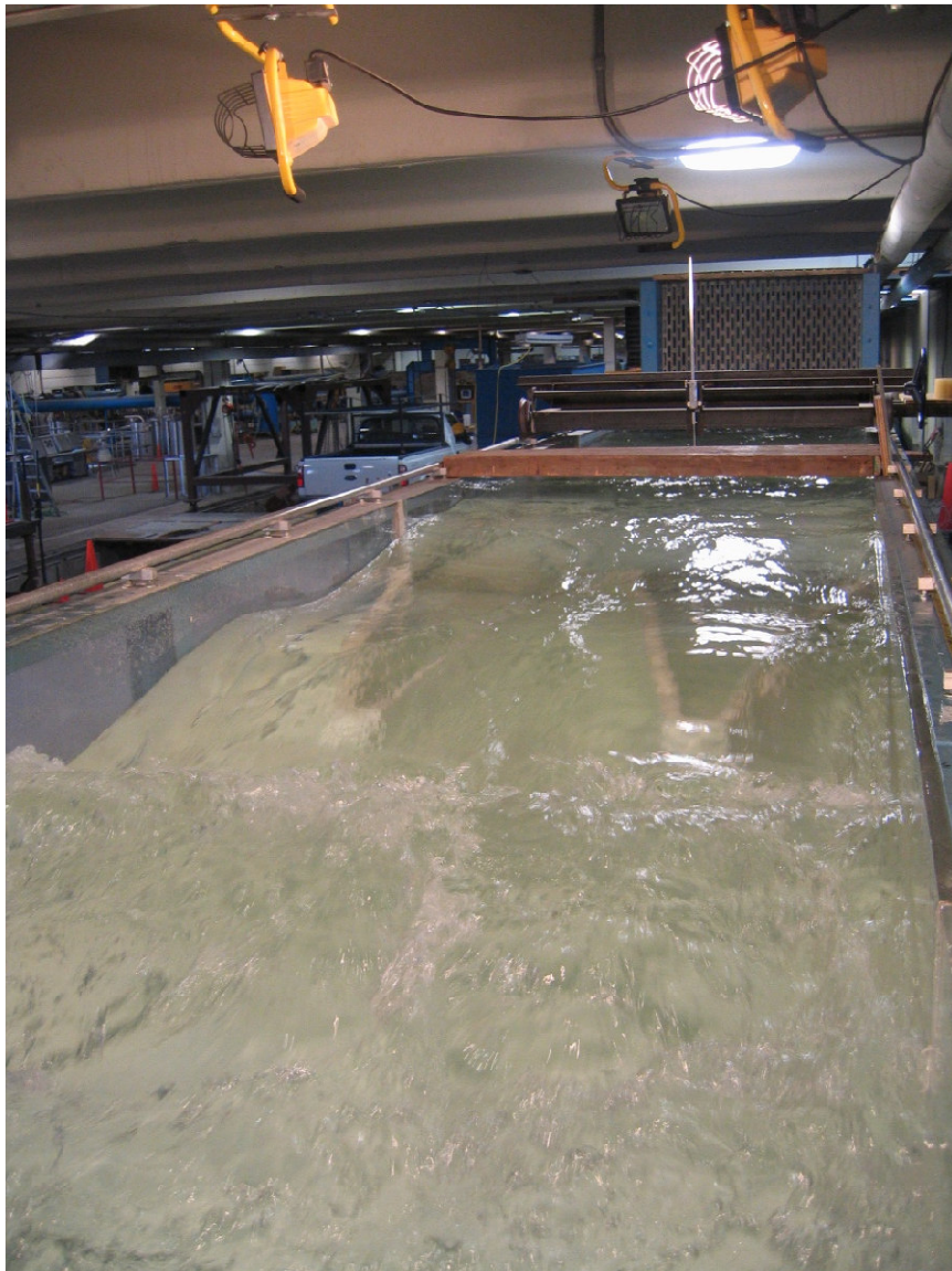
Fig. 3-21. Tailwater submergence for the 10° half-round trapezoidal labyrinth weir
