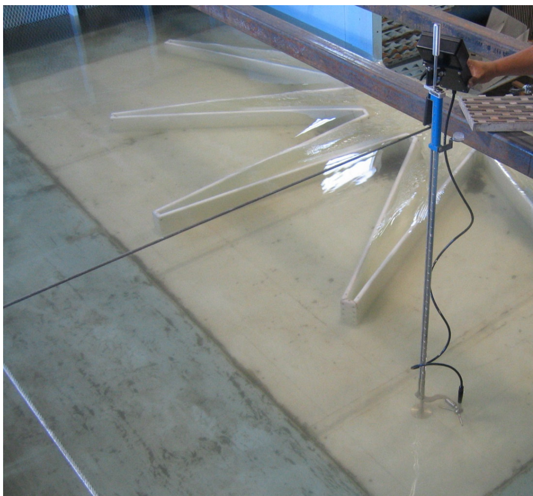
Fig. 3-14. Velocity field mapping with 2-D acoustic doppler velocimeter
