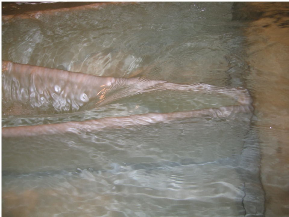
Fig. 3-22. Local submergence at an upstream labyrinth apex
