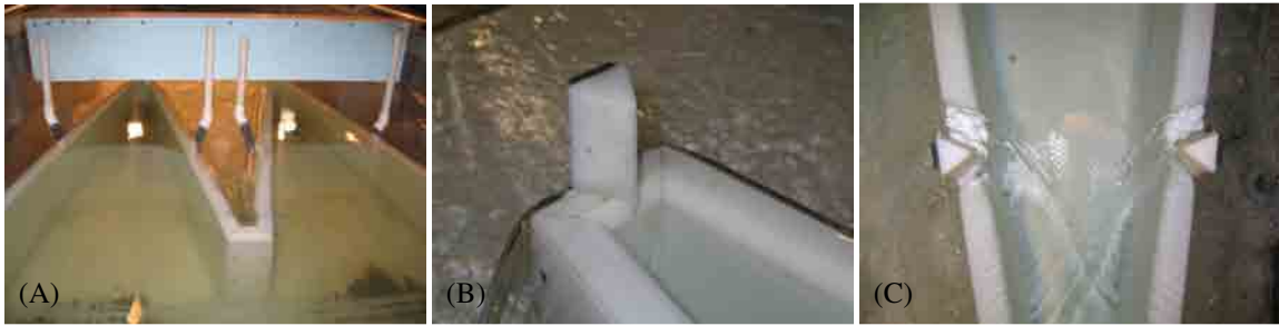
Fig. 3-18. Aeration tube apparatus for N = 2 (A) and nappe breakers located on the downstream apex (B) and on the sidewall (C)
