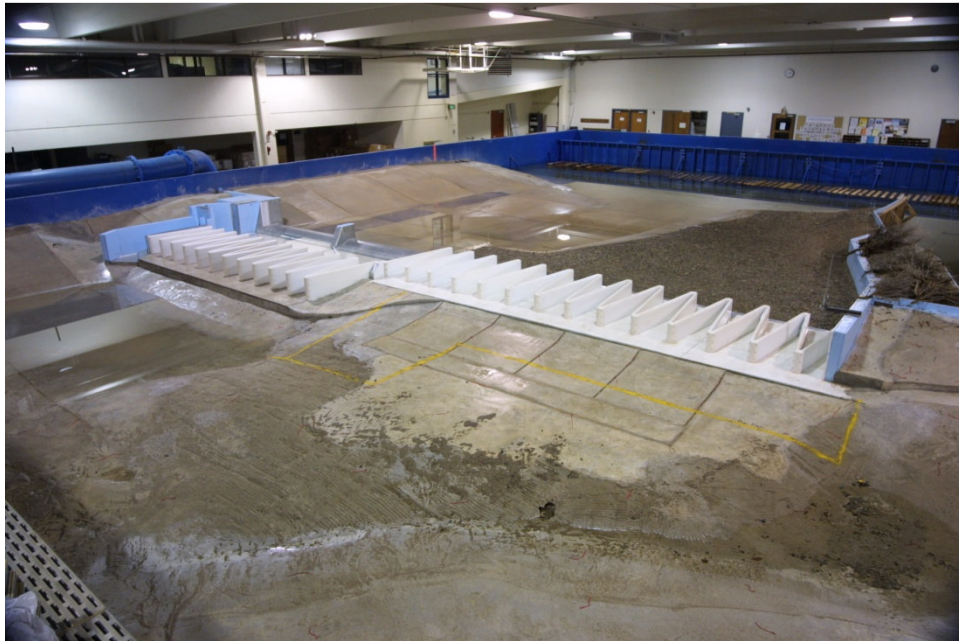
Fig. 2-14. Full-width model of Lake Brazos labyrinth spillway in Waco, Texas, USA
