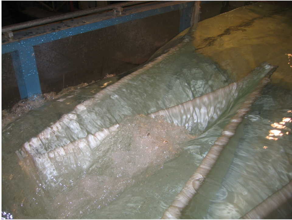
Fig. 3-23. A labyrinth standing wave in the downstream cycle
