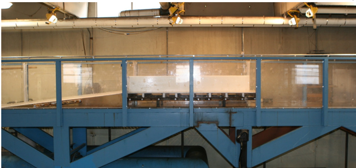
Fig. 3-2. Rectangular flume test facility
