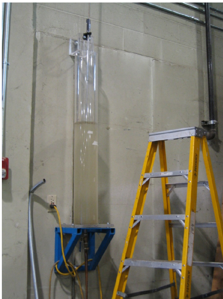
Fig. 3-11. Stilling well used for the reservoir test facility
