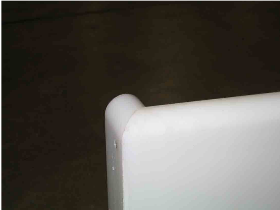
Fig. 3-16. The joint between the \frac{1}{2} apex (to be attached to flume wall) and the weir sidewall of the 2-cycle, 6^\circ half-round labyrinth
