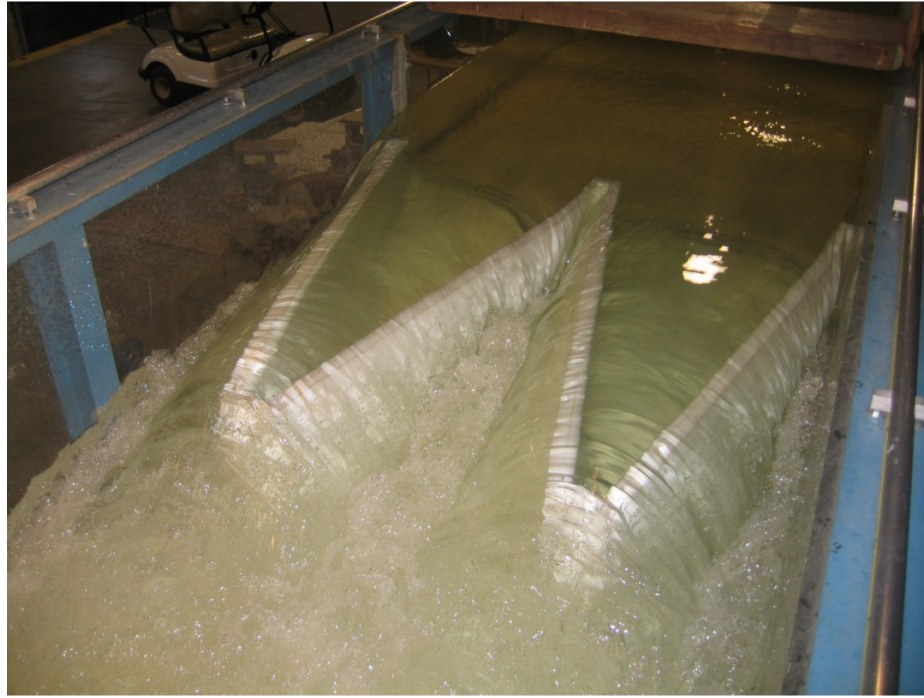
Fig. 6-10. Drowned nappe aeration condition observed for trapezoidal labyrinth weir, quarter-round crest shape, \alpha = 12^\circ , H_T/P = 0.604
