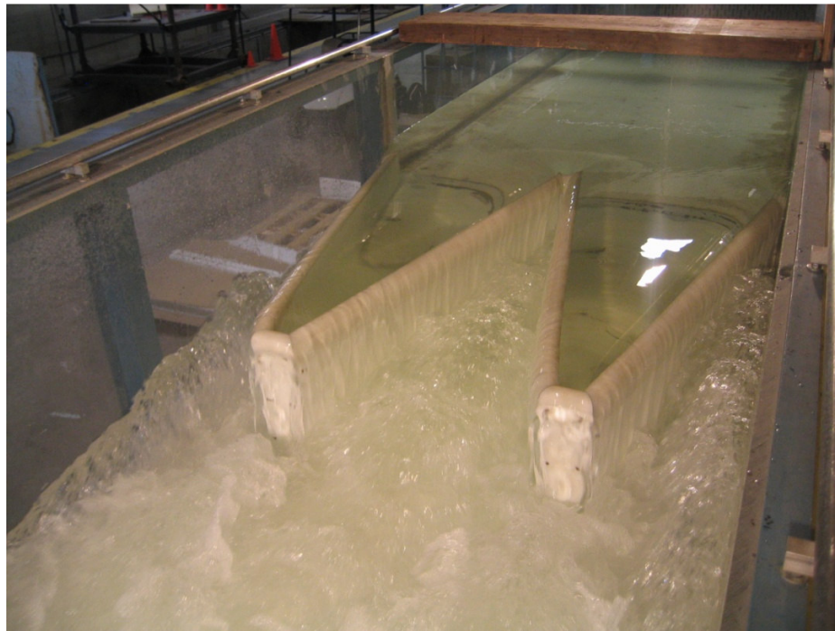
Fig. 6-7. Clinging nappe aeration condition observed for trapezoidal labyrinth weir, half-round crest shape, \alpha = 12^\circ , H_T/P = 0.196
