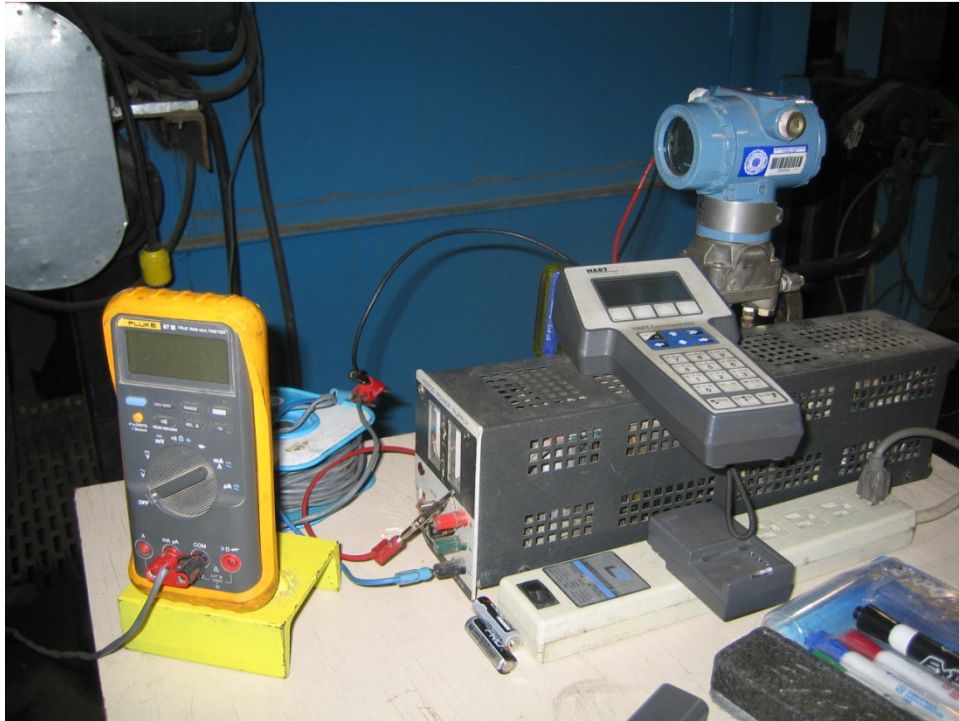
Fig. 3-9. Flow measurement equipment (power supply, pressure transducer, data logger, and Hart communicator)
