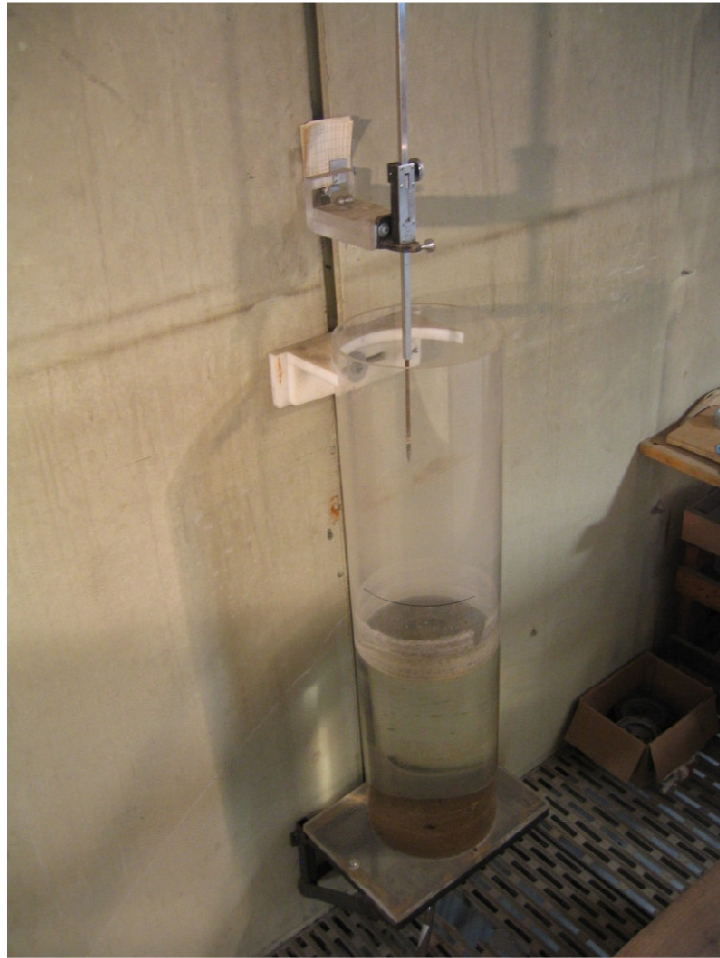
Fig. 3-10. Stilling well used for the rectangular flume facility
