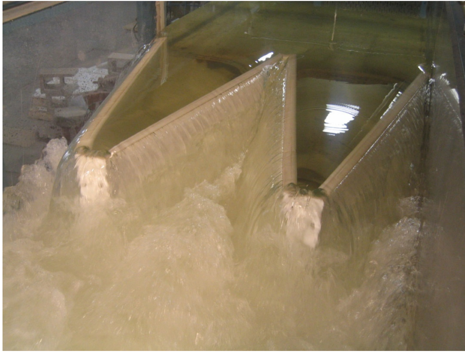
Fig. 6-8. Aerated nappe aeration condition observed for trapezoidal labyrinth weir, quarter-round crest shape, \alpha = 12^\circ , H_T/P = 0.202
