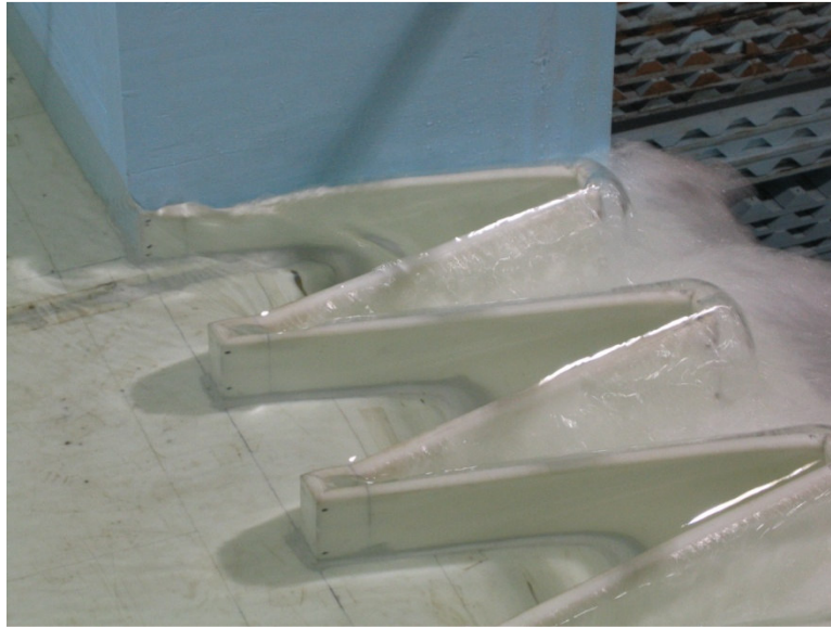
Fig. 6-1. Example of a labyrinth weir
