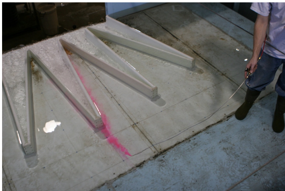
Fig. 3-15. Flow pattern and direction observations with the dye wand
