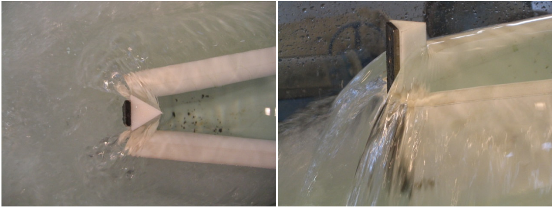
Fig. 4-7. Wedge-shaped nappe breakers placed on the downstream apex
