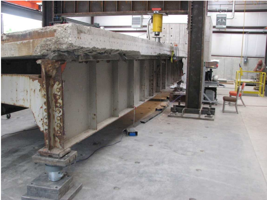
Figure 6. Specimen 1 beneath reaction frame.
