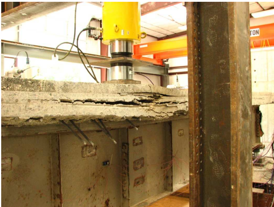
Figure 34. Flexural cracks after a) 1,420 kN (320 k ) and b) failure, 1,490 (334 k ).
