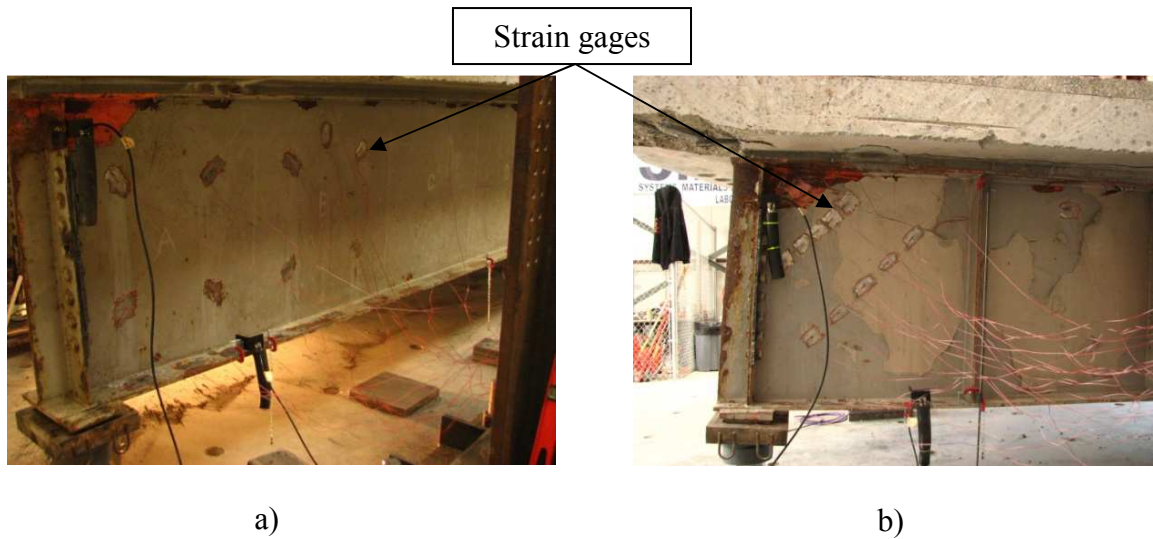
Figure 19. Strain gage configuration for Beam Shear Tests a) B and b) c.
