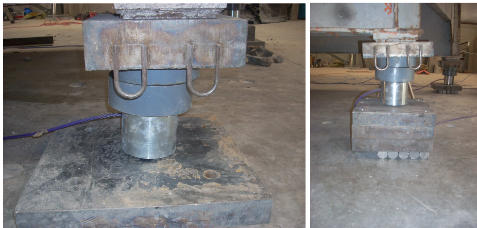
Figure 7. a) Eccentric loading of load cell and b) roller reaction.
