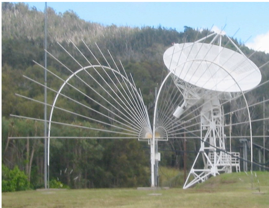
Figure 3.3: Palehua's 28-ft dish is used to monitor 245, 410, and 610 MHz radio emissions from the sun. This picture shows the old tracking mechanism, that was replaced in late 2007.
