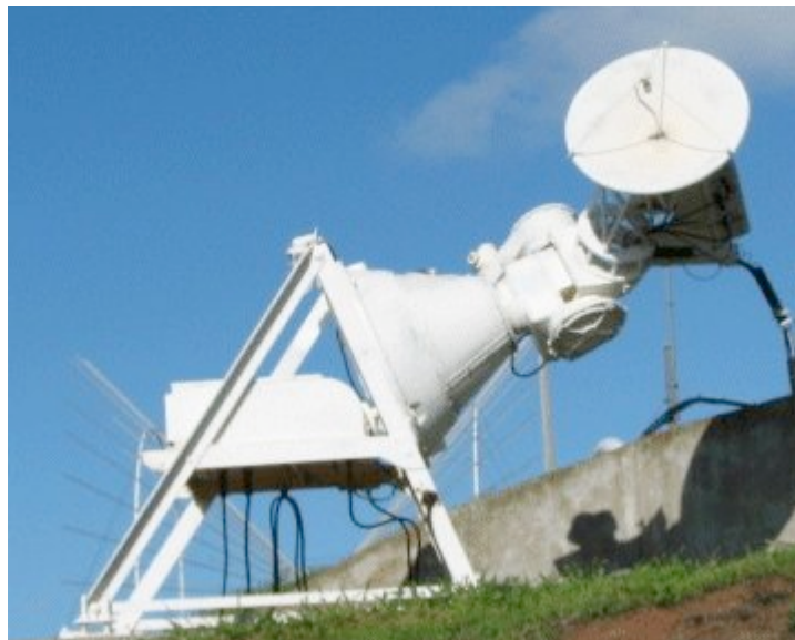
Figure 3.5: 3-ft parabolic dish antenna at Palehua Solar Observatory is used to monitor 15,400 MHz. The antenna is mounted on top of the tracking mechanism.
