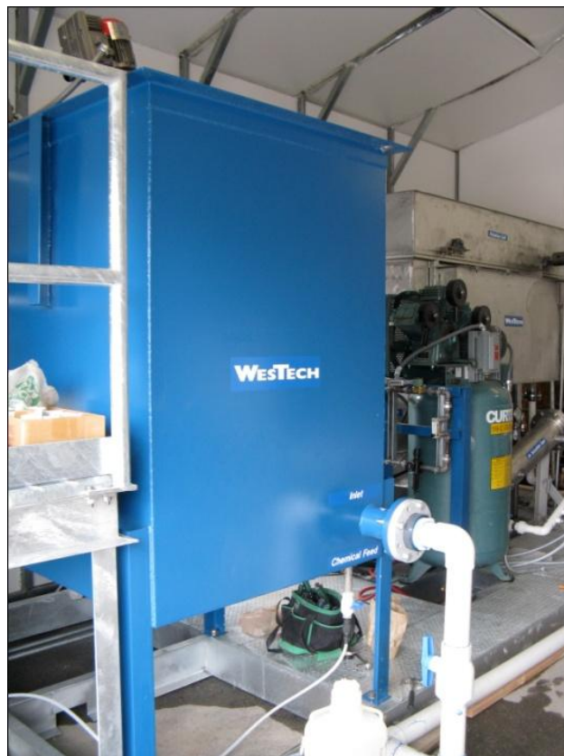
Fig. 11. Flocculation tanks on pilot DAF unit
