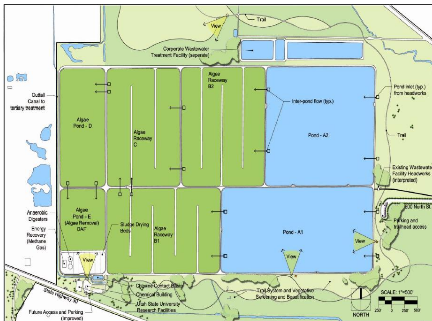
Fig. 6. Potential Logan Lagoons flow diagram
