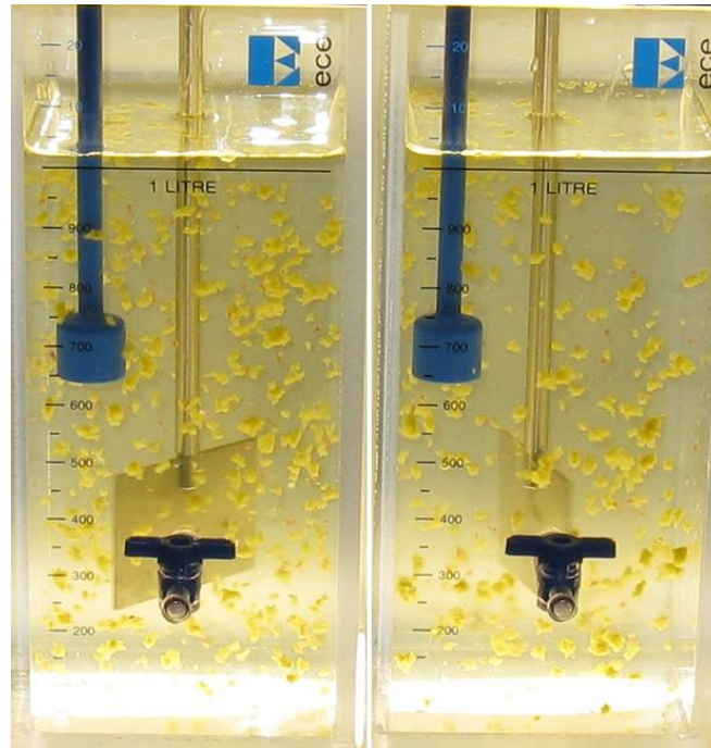
Fig. 46. Algal flocculation in jar test unit; 30 mg/L alum with 0.6 mg/L polymer (left) and 30 mg/L alum with 1.0 mg/L polymer (right)
