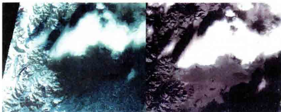
FIGURE 6.28. Cloud and Snow Separation Using Landsat Band 7 (04/01/2000). False Color (left) and Band 7 (right) Showing Contrasting Reflection.
