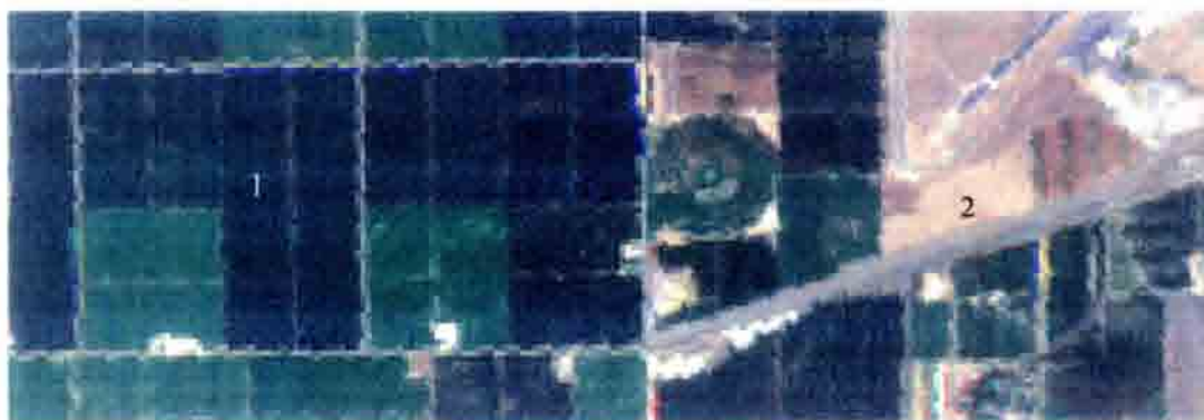
FIGURE 6.4. Approximate Location of the Cold (1) and Hot (2) Pixels for a Landsat 7 ETM+ Scene (shown in true color) for 07/12/2002. The Cold Pixel Is in a Full-Cover Alfalfa Field, and the Hot Pixel Is in a Bare and Dry, Agricultural Field
