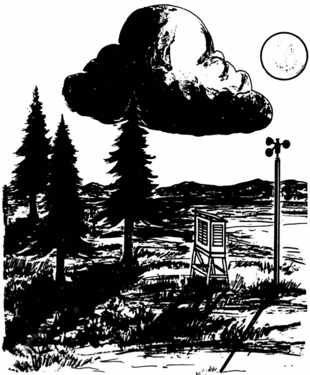
Figure 2.—Environmental conditions influencing fuels subject to solar heating are not measured by instruments in weather shelter.
