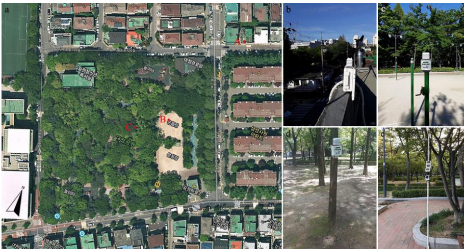
Figure 2. In-situ measurements: a) aerial view of Daecheong Park; b) sampling point A; c) sampling point B; d) sampling point C; e) mobile measurement: one GPS and three TR-72wf Thermo Recorders were attached to a metal pole at 0.1, 1.5, and 2 m above the ground
