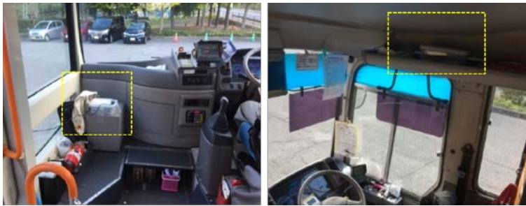
Figure 4. Installing WiFi Scanner on Bus No.1 and Bus No.2
