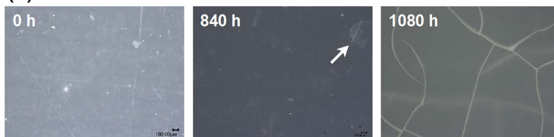
Fig. 1 (a) Macroscopic and (b) microscopic images of the LDPE sheets before and after UV irradiation. The exposure times are shown in the figures. The arrow denotes the onset of surface crack formation.
