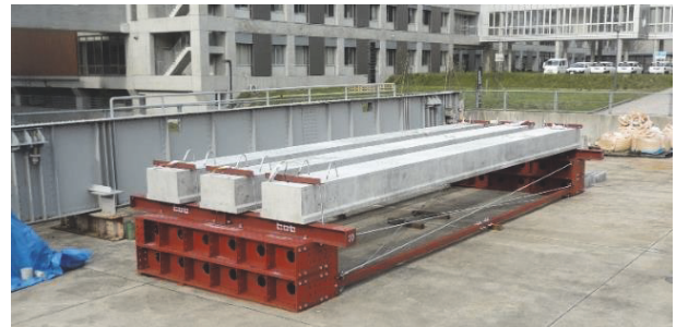
FIGURE 2: PC girders constructed for this study.
