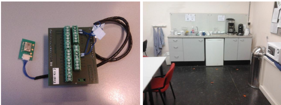
(a) Thermopile sensor used: GridEye. (b) For evaluation about office pantry area.
