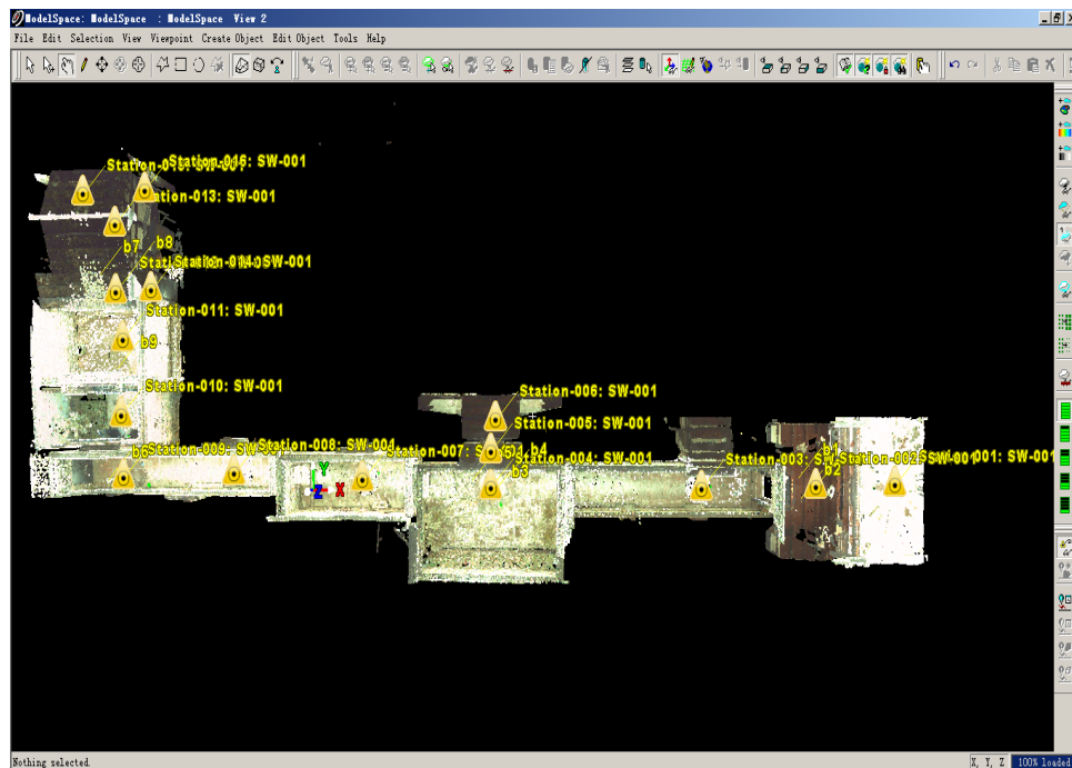
Figure 2-4 The measuring sites and measuring targets
