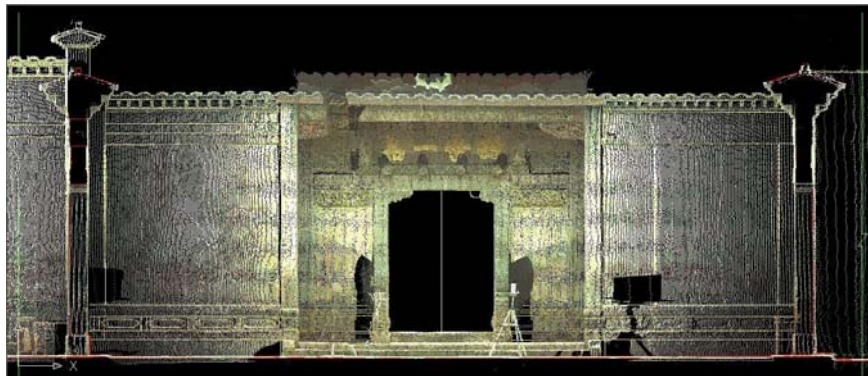
Figure 2-6 The drawing of the entrance vertical face section from the point clouds
