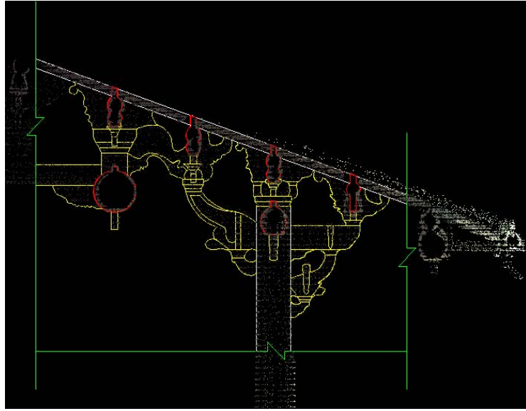
Figure 2-14 The drawing of the Dougong beams above the Gold Pillar using the point clouds
