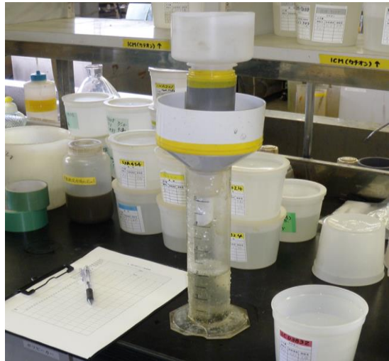
Figure 3.3 Simple gravity filtration measuring device
