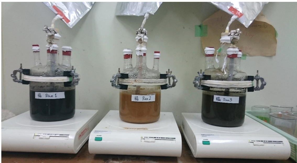
Figure 4.1 Reactors used in the continuous experiment
