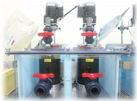
Figure 2.4 Reactors used in lab-scale co-digestion experiment
