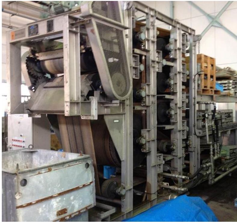
Figure 3.5 Belt press used in the dewatering experiment
