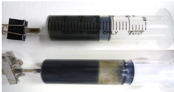
Figure 3.1 Syringes used as digesters in the batch experiment
