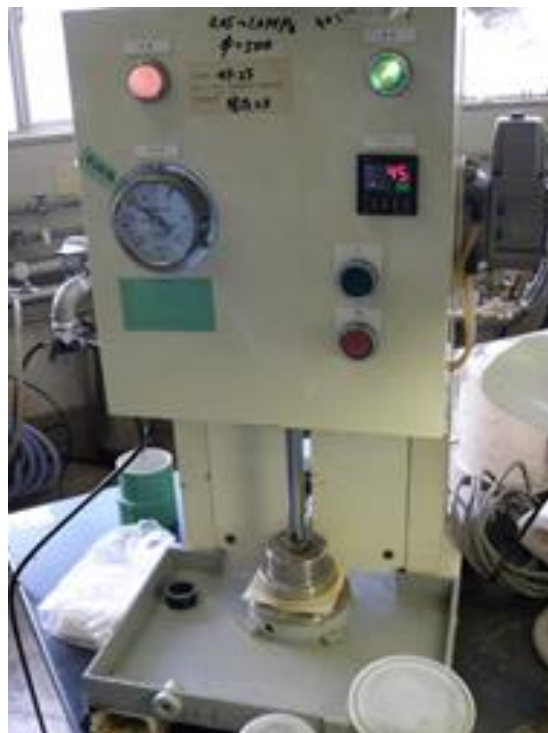
Figure 3.4 Simple dewatering tester used in the coagulant selection test
