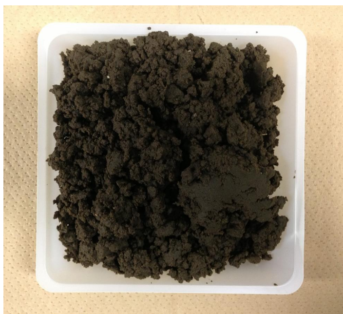
Figure 2.2 Dewatered oxidation ditch sludge
