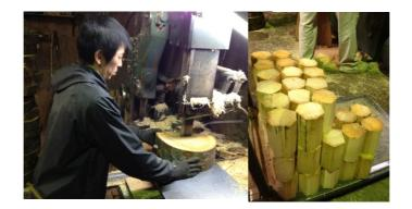
3. Wood turning, consists of rough turning and finishing turning
