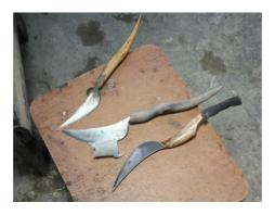
Small knives for cut and slicing bamboo
