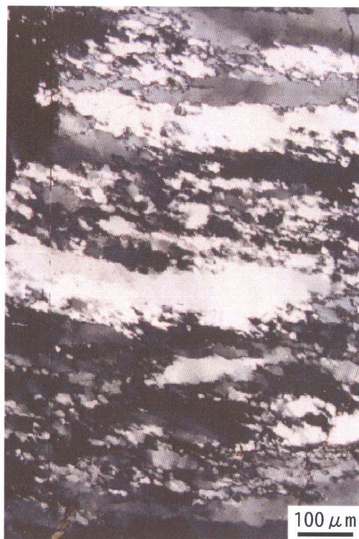
Fig. 2 Optical micrograph (crossed polarizers) showing the representative microstructures of the studied quartz aggregates in a mylonite collected from Hatagawa shear zone.
