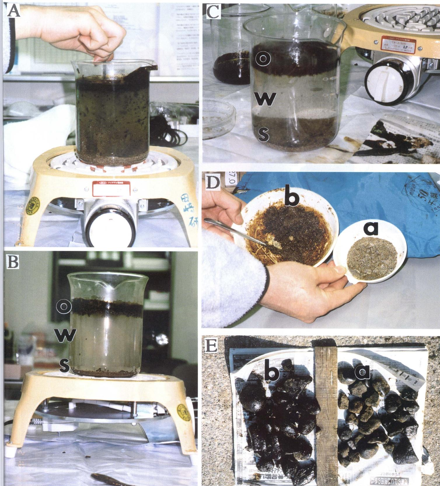
**Figure 18** Separation experiments of C – typed heavy oil and sands or gravels by warmed seawater. O; oil, W; water, S; sands, b; before, a; after.
