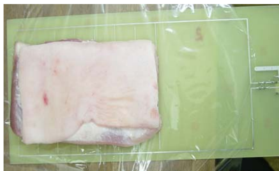
Figure 1. The interdigital sensor and pork belly cuts
