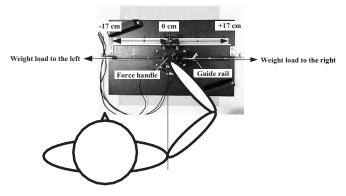
Figure 1. The experimental instrument and setup seen from the upper surface
