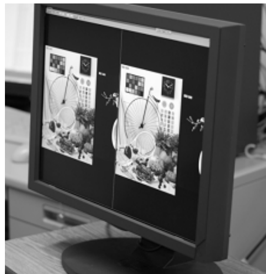
Fig.4. The newly developed resolution-enhanced 9MP LCD (TOTOKU ME351i base)
