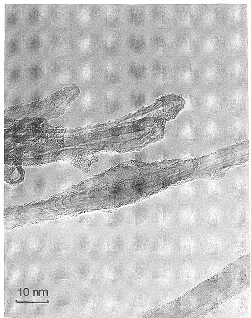
Fig. 8. Electron micrograph of a nanoparticle similar to the tips of nanotubes. The nanoparticle, which overlaps the nanotube, is found in the soot in the tungsten basket heater.
