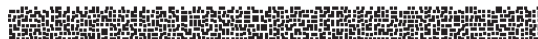
Fig. 4. Jaggies that appears in the horizontal lines when pseudorandom pixel placement is applied.
