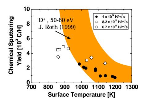
Fig. 4 Temperature dependence of chemical sputtering yield estimated by the weight loss of graphite targets.
