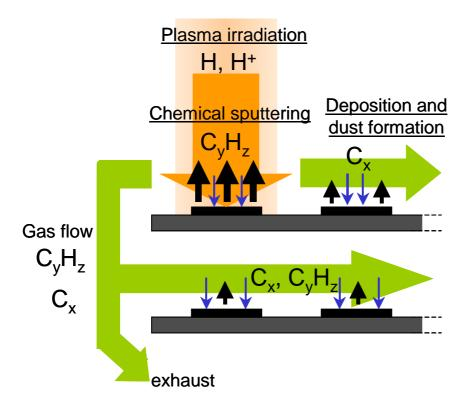
Fig. 7 Schematic illustration of erosion and dust formation in the present experiments Scale figure size: Single (75 mm) journal column width
