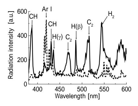
Fig. 3 Radiation spectra from the plasma at 5 mm above graphite target 1 during Ar (dotted line) and  $Ar/H_2$  (solid line) plasma irradiation.
