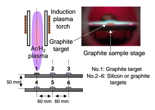
Fig. 1 Schematic diagram of atomic hydrogen irradiation system using high power ICP.
