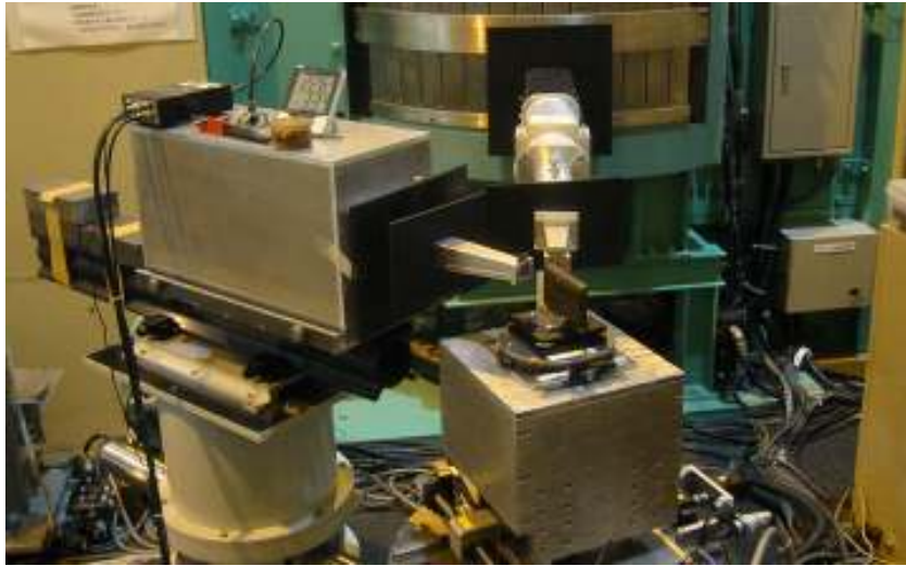
Fig. 2, Example of experimental set-up for neutron stress measurement of lattice spacing in transverse direction with RESA.
