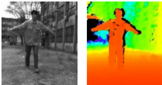
Fig.3. Example of disparity image. Left-side image is a original image and right-side image denoted a disparity image corresponding to left-side image. In this disparity image, brightness shows distance from camera, it is shown that the brighter, the shorter the distance is.
