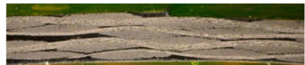
(b) Top part with no voids in case of 0.2mm additional stroke Fig.19 Effect of additional stroke on the inside structure
