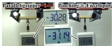
Figure 16. Results for feasibility test to evaluate whether the maximum weight of graspable objects is more than 3 kg
