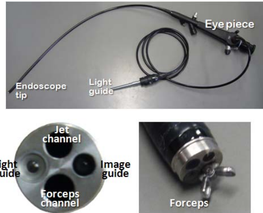
Fig. 2 Photographs of the newly designed endoscope
