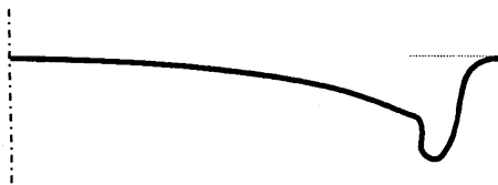
Fig. 15 Deformed shell when buckling
