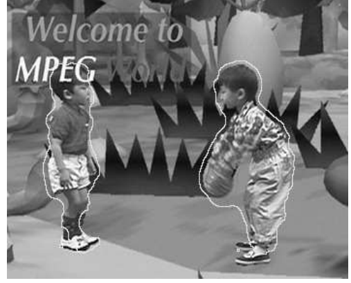
Figure 2. Extraction from the Frame Difference with the LoG Filter.
