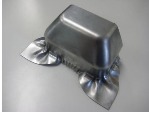
Fig.7 Wrinkling in experiment
