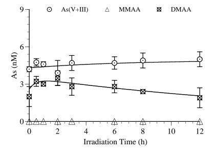
Fig. 3: Effect of irradiation time with a 400 W high-pressure mercury lamp on arsenic speciation in filtered water sample. Samples were collected from surface level of Lake Kiba on 25 May, 2006. Error bars represent mean  $\pm$  S.D.
