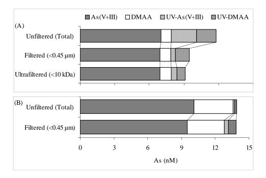
Fig. 5: Mean concentration and distribution of arsenic in surface water (depth 0 m) of Lake Kiba (A), and Lake Biwa (B) collected on 31 Jul., 2006 and 29 Jul., 2006, respectively.
