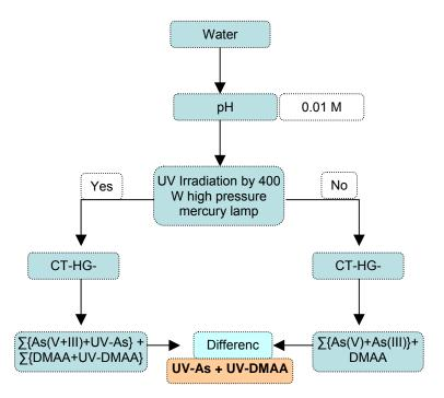
Fig. 1: Schematic diagram showing the protocol for the determination of ultraviolet-labile fractions (UV-As and UV-DMAA) of arsenic in Lake water following UV-Irradiation.
