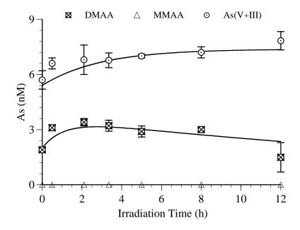
Fig. 2: Effect of irradiation time with a 400 W high-pressure mercury lamp on arsenic speciation in unfiltered water sample. Samples were collected from surface level of Lake Kiba on May 25, 2006. Error bars represent mean  $\pm$  S.D.
