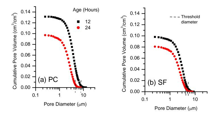
Fig.2 Coarse capillary pore size distributions at early ages (a) Portland cement concrete (b) Silica fume-containing concrete
