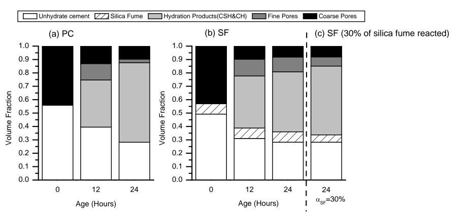
Fig.3 Volume fractions of constituent phases in concretes (Coarse pores :> $0.2\mu$ m, Fine pores: $0.2\mu$ m-2.5nm)
