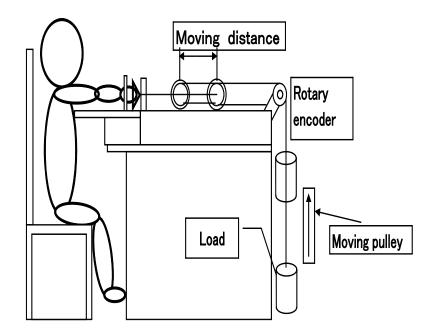
Figure1. Scheme of measurement device. The device consists of grip handle, rotary encoder attached at the fixed pulley, and variable load. These connect by moving pulley and wire. The rotary encoder can measure the rotational angle when the load was pulled up by hand grip movement.
