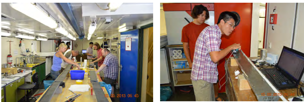
Fig. 3.4: Cutting (left) and color scanning (right) of the Gravity cores in the Geo-lab.
