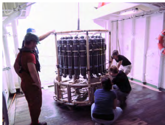
Fig. 4.2: Removing the turbidity sensor.
