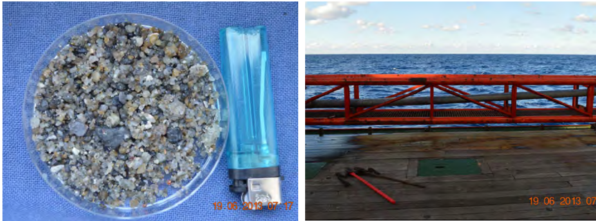
Fig. 3.5: sample material collected from the core-catcher at GeoB 17438 (left), where the tube was bent (right).
