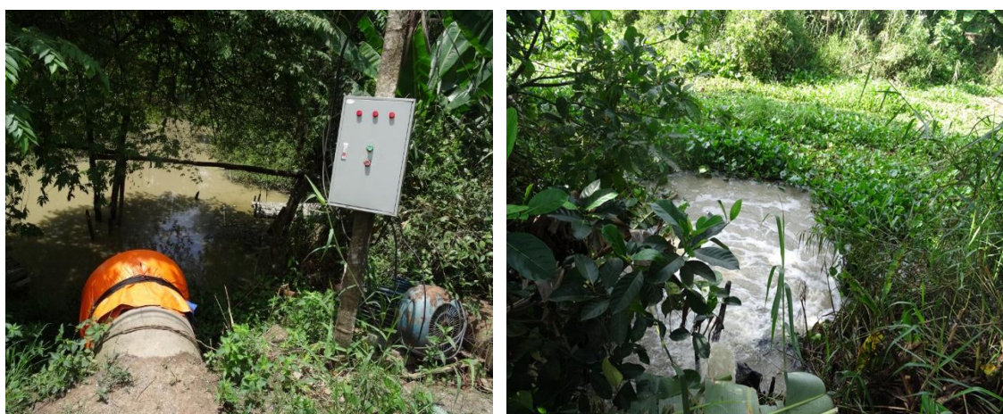
Figure 5.10: Collective draining water from a large rice farm to a public canal in the rainy season in Vinh Trach commune Source: Author (2016)
