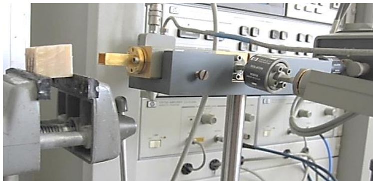
Fig. 40: Set up of VNA test of aging samples in reflection mode
