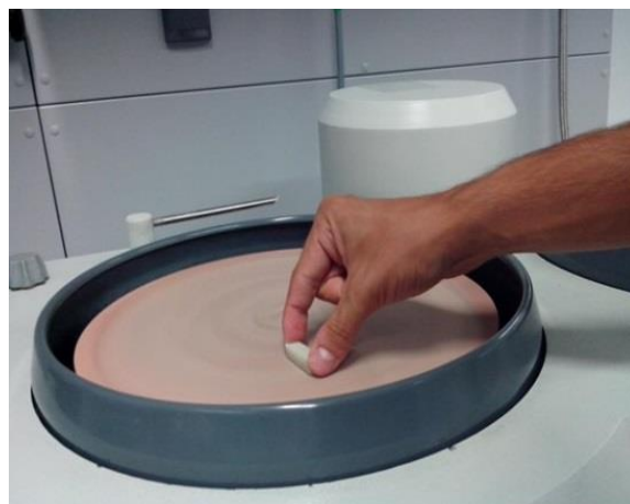
Fig. 36: Polishing of CIPP sample
