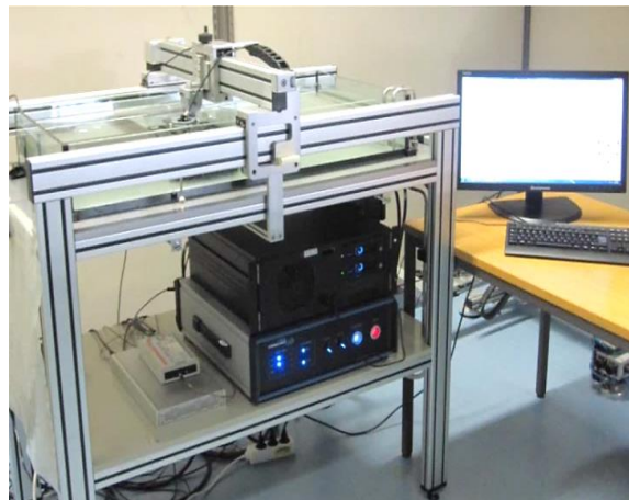
Fig. 32: The ultrasound system specified and constructed by the company I-Deal
