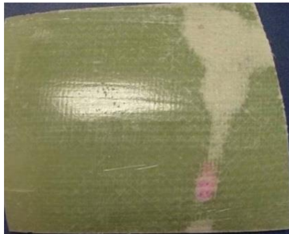
Fig. 9: Discoloration of liner due to insufficient curing [Bosseler 2009]
