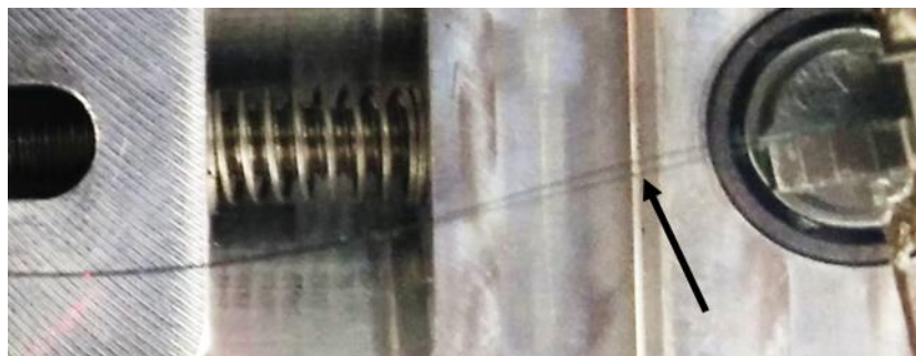
Figure 4.30: Stack of two 50 \mu\text{m} thick bi-stable springs. An apparent gap between the two springs resulting from the different distance to the pivot point can be observed.
