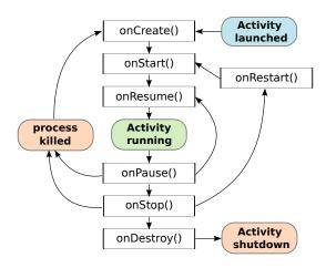
Figure 2.2: Activity lifecycle (adapted from (48)) with predefined callback methods.
