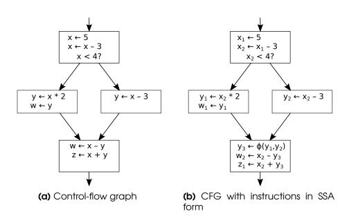
Figure 2.3: Control-flow graph with original instructions and instructions in SSA form.
