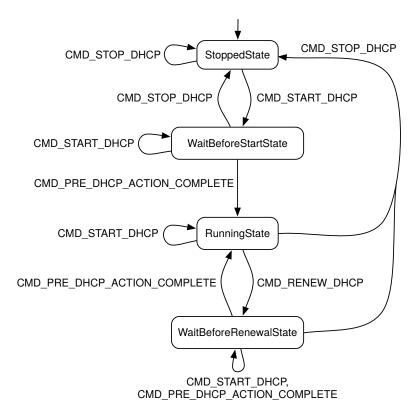
**Figure 4.1:** Simplified DHCP state machine from class android.net.DhcpStateMachine~ . Omitted commands do not cause state transitions. States provided by the default implementation (halting and quitting) are not shown.
