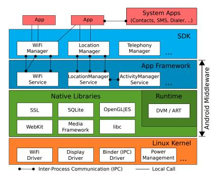
**Figure 2.1:** Android Software Stack with six different layers. Some IPC and local calls are depicted to exemplify different communication pattern across layers.
