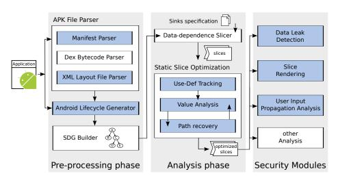
Figure 3.1: High-level architecture of R-DROID
