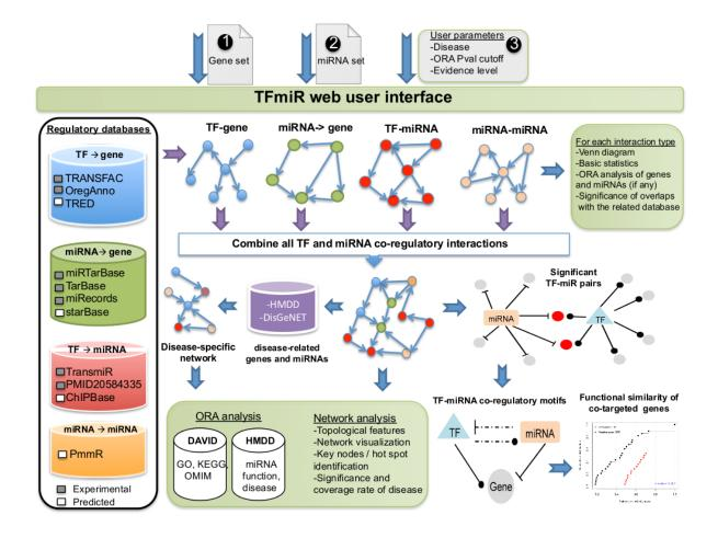
Figure 4.1: A system level overview of the TFmiR architecture describing the incorporated databases, data flows and output downstream analysis.
