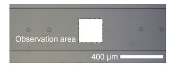
FIGURE 4.3 – Light microscope image of the microfluidic channel and the observed area (white). MTB were redirected before drifting out of the center of the field of view.
