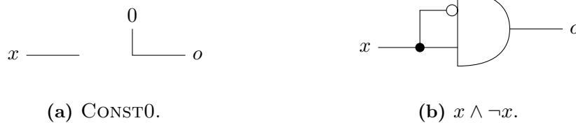
Figure 4.5: Two combinational logic DAGs implementing x \mapsto 0 (a) and x \mapsto x \wedge \neg x (b). While these are equivalent w.r.t. Boolean logic, i.e., under stable inputs, they are not equivalent w.r.t. Kleene logic, i.e., under metastable inputs.
